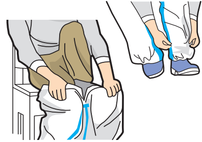
Remove shoes and secure trousers into socks. Step into legs of coverall and place coverall over safety boots.
